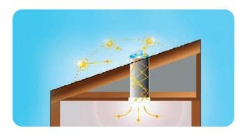
This Eco friendly system is designed to capture natural light and directs it through tubes internally quoted with highly reflective material thereby minimizing the dispersion of the rays. This supply lights to considerable distance without Heat or cold transfer.
